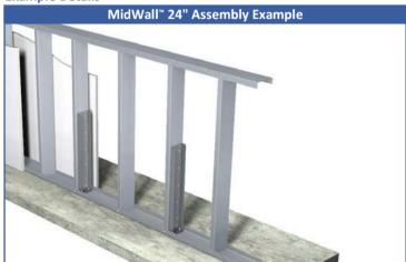
Midwall™ 24" is generally used in interior half walls of less than 48" in height. Attach Midwall to 54 mil stud with #12 screws through all pre-drilled guide holes. Other studs in the wall are typical infill studs.
