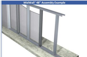
Midwall™ 48" is used in interior half walls equal to or more than 48" in height. Use one Midwall 48" as a substitute for a stud at the specified spacing, or attach to a 54 mil stud with #12 screws through all pre-drilled guide holes.
