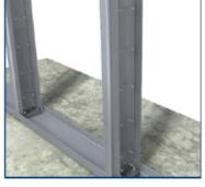
Attach 24" Midwall to the stud web with #12 screws fasteners through guide holes in vertical leg.
